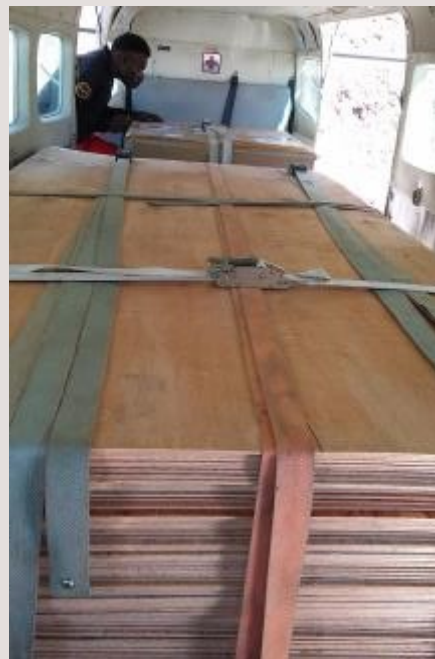
Plywood well strapped down
