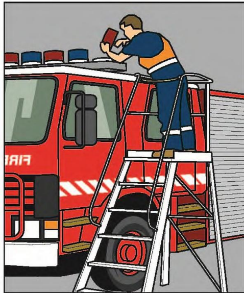
Figure: A step platform can provide a stable work surface
